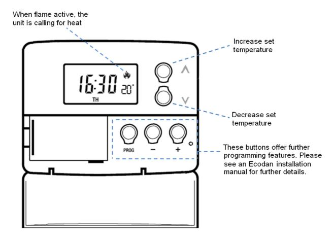
A thermostat measures the room temperature and activates the heating system to maintain the desired temperature.
